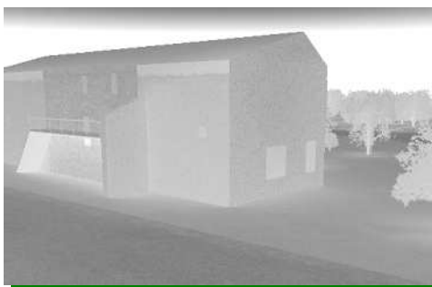
LWIR signal taking into account the global illumination of a cloudy sky.
